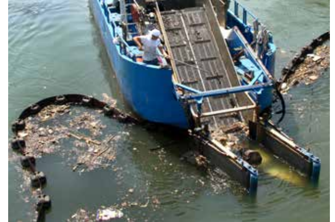
Using more trash booms in the Creek will help us remove floating garbage. Photo: Charles Denson
